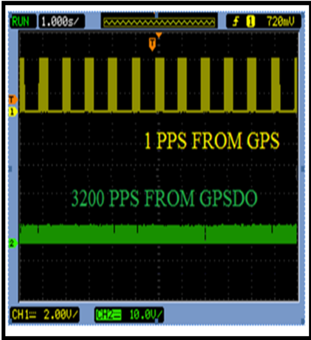
Fig. 6. 1 PPS from GPS and Respective output pulses of GPSDO In the fig. 6 it is shown that the 1PPS is converted into required number of pulses(3200). For clear observation it is shown in Fig.7.
